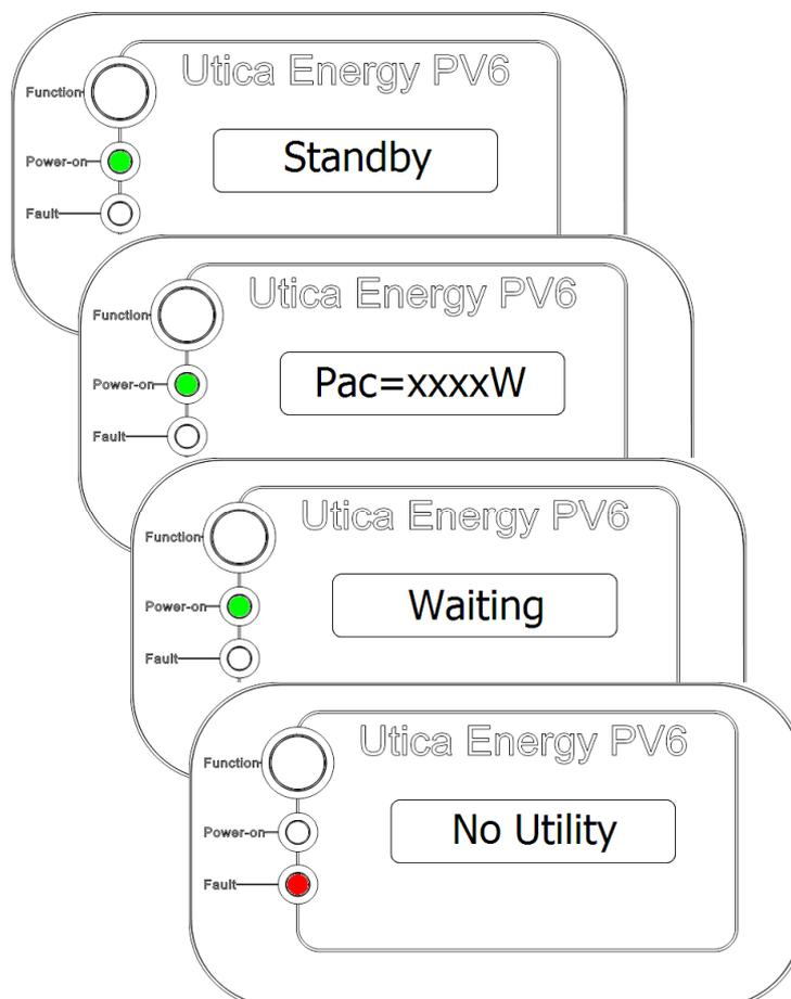
(2) Close the AC breaker or fuse between the PV Inverter and the grid. The PV Inverter status should change to normal operation after a countdown "Checking xxS" if the PV array is energizing with a DC voltage higher than 180VDC.
