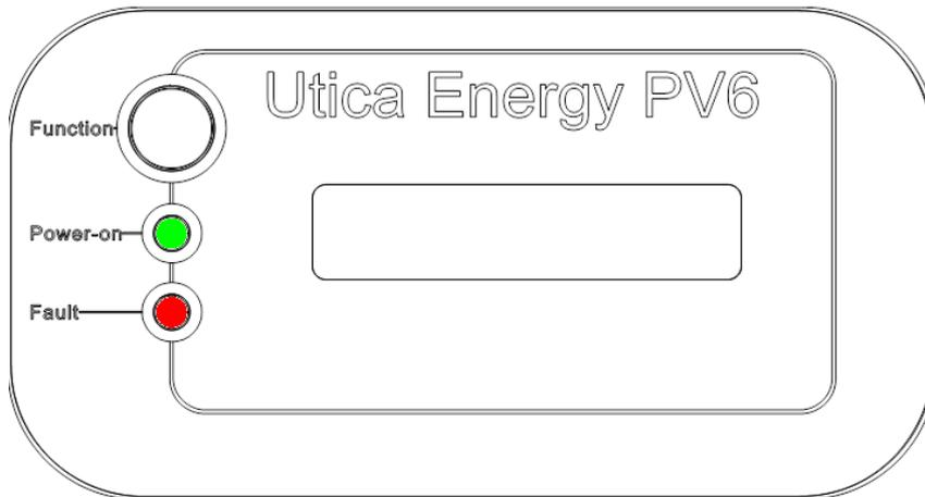
When the PV array is connected and the input voltage is higher than 180VDC, if the AC grid is not connected the LCD will display the following message "Standby" -> "XXXX W" -> "Waiting" -> "No Utility". In this status the "No Utility" message will remain and the RED Fault LED is illuminated.
