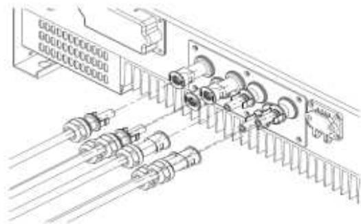
(2) Use MC4 or compatibly MC4 (Multi-contact®) connectors for the DC wiring. (ex: Wieland PST40il)
